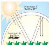
Infrared retains thermal energy
