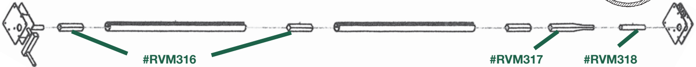
Diagram above shows order of installation of E-ZY Grower Roll Tube with adapters into guide and gear box.
