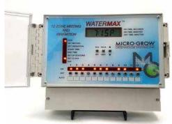
Time-based irrigation and misting control system. Twelve individual stations may be individually set for operation times, watering days, and repeat functions. The propagation mist adjustments include separate start and stop times, as well as on and off times for complete mist cycle operations.
